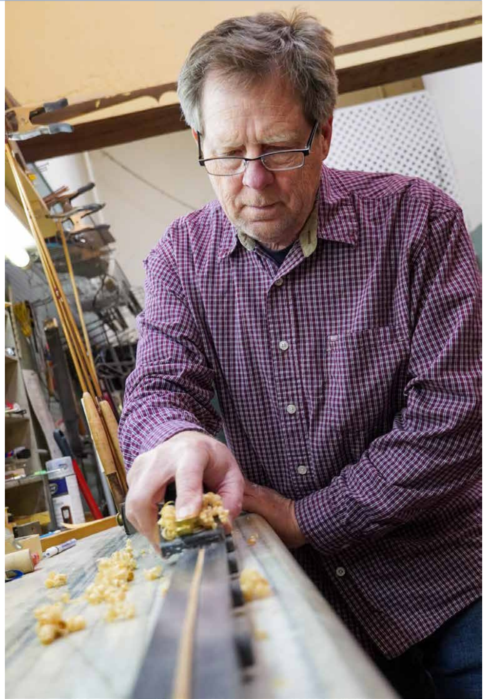
STEVE SOBIENIAK PLANES A STRIP OF TONKIN CANE IN THE PROCESS OF MAKING A NEW BAMBOO ROD.
